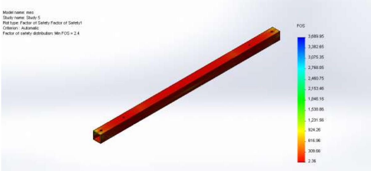
Figure - 4.2.6: Factor of safety of axle for SAE 304 material.
